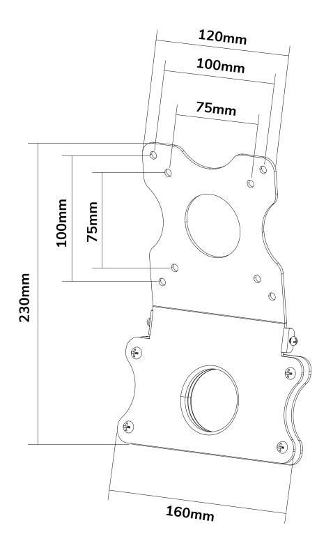
Neomounts Measuring unit: mm
